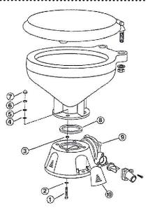
positioned in its groove (a little grease may be used to hold it in place) and carefully (so as not to dislodge the seal) slide the pump assembly into the base. Secure the pump to the base with the four machine screws and lock washers and torque each to 13-15 inch pounds.
